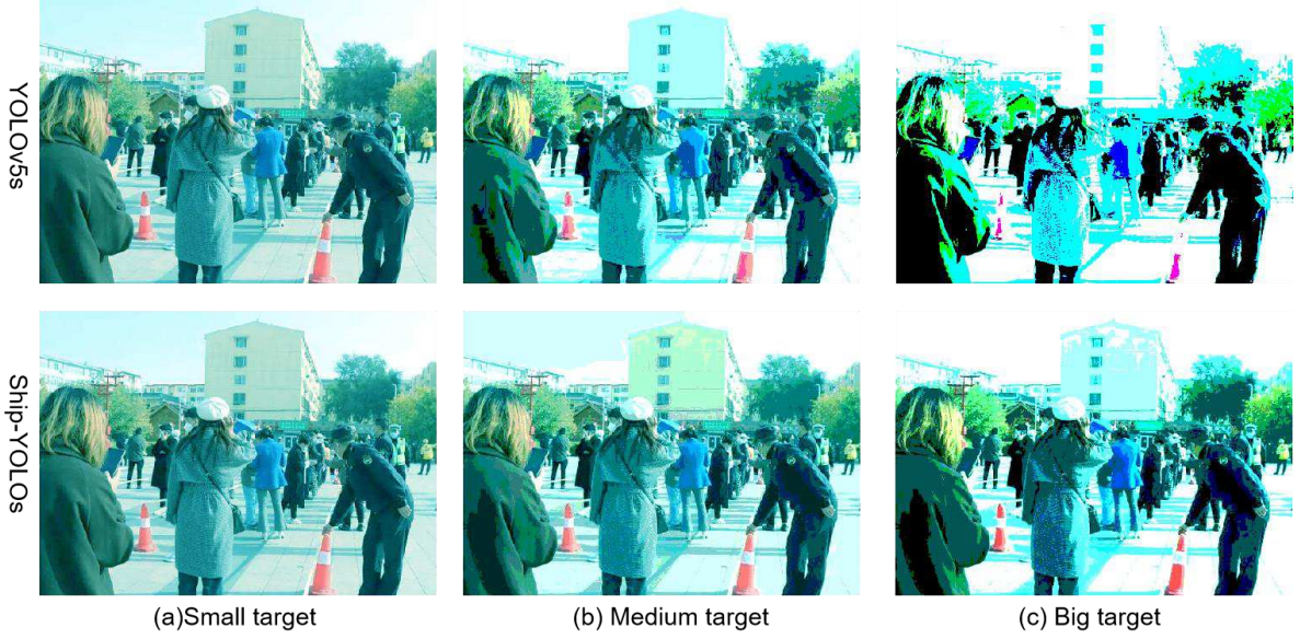
Fig.8 The thermal maps of the feature maps for the detection of different size target in the detection head based on the confidence degree
