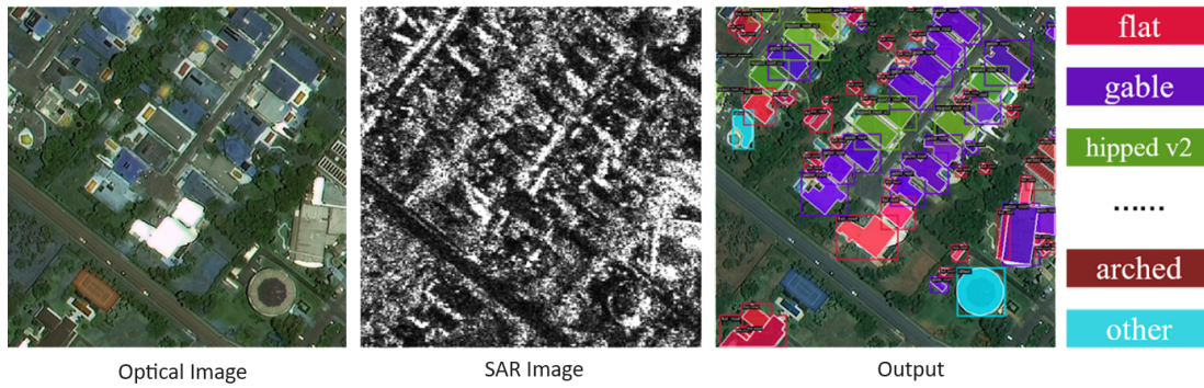
Fig. 1: Example image tile of the provided multi-modal data (optical and SAR) for building detection and roof type classification.
