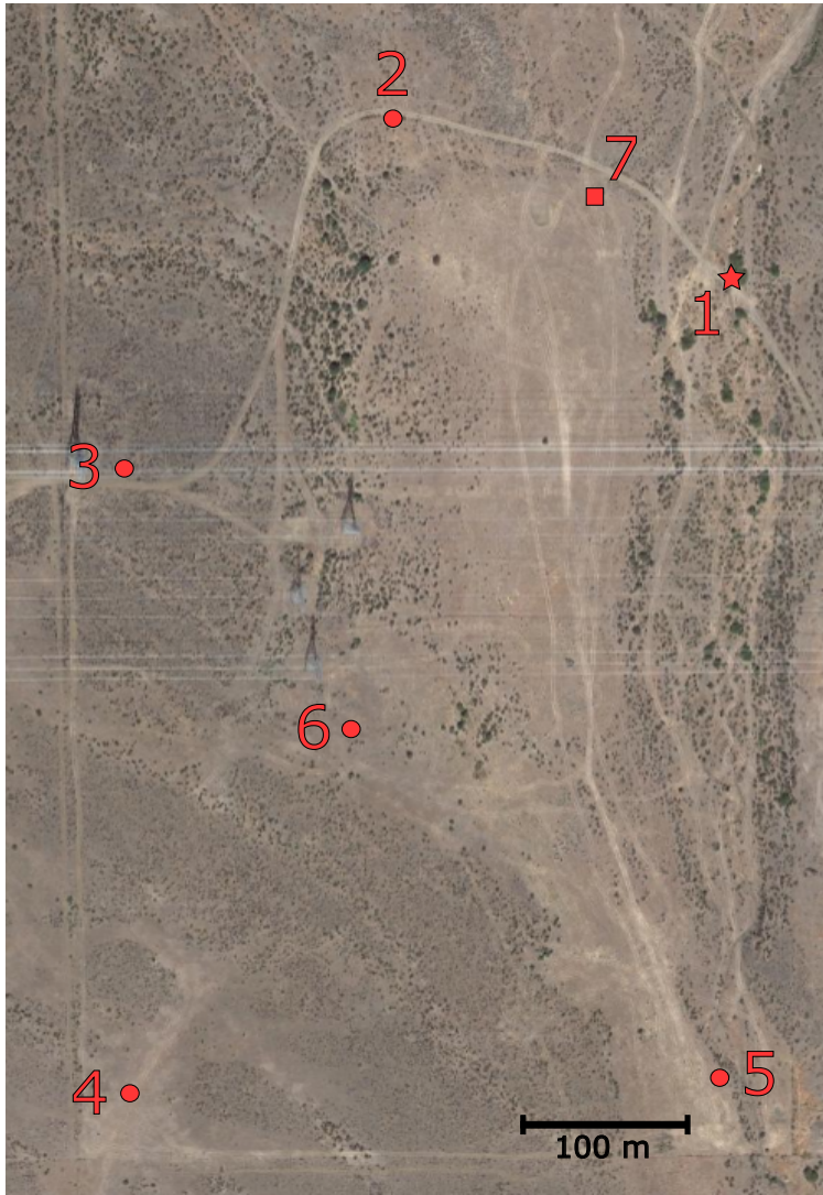
Fig. 7: Complex courses Tour (left) and Baja (right) with numbered and alphabetized waypoints. The Tour is approximately two kilometers in total distance with \pm 80 m of elevation change. Reaching waypoints 4 through 7 require traversal of steep slopes and ditches. Waypoints I through 4 test trail-following and nominal behaviors (obstacle avoidance and basic navigation and control). Baja is approximately three kilometers and repeatedly crosses the region densest in ditches and vegetation from waypoints E through U .
