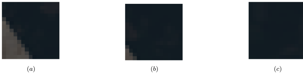
Figure 8. A non-boundary (negative) patch where the centre pixel is not a boundary pixel – enlarged for visualization purposes – extracted at different scales; (a) 59 \times 59 downsampled to 15 \times 15 (coarse), (b) 29 \times 29 downsampled to 15 \times 15 , (c) 15 \times 15 (fine).
