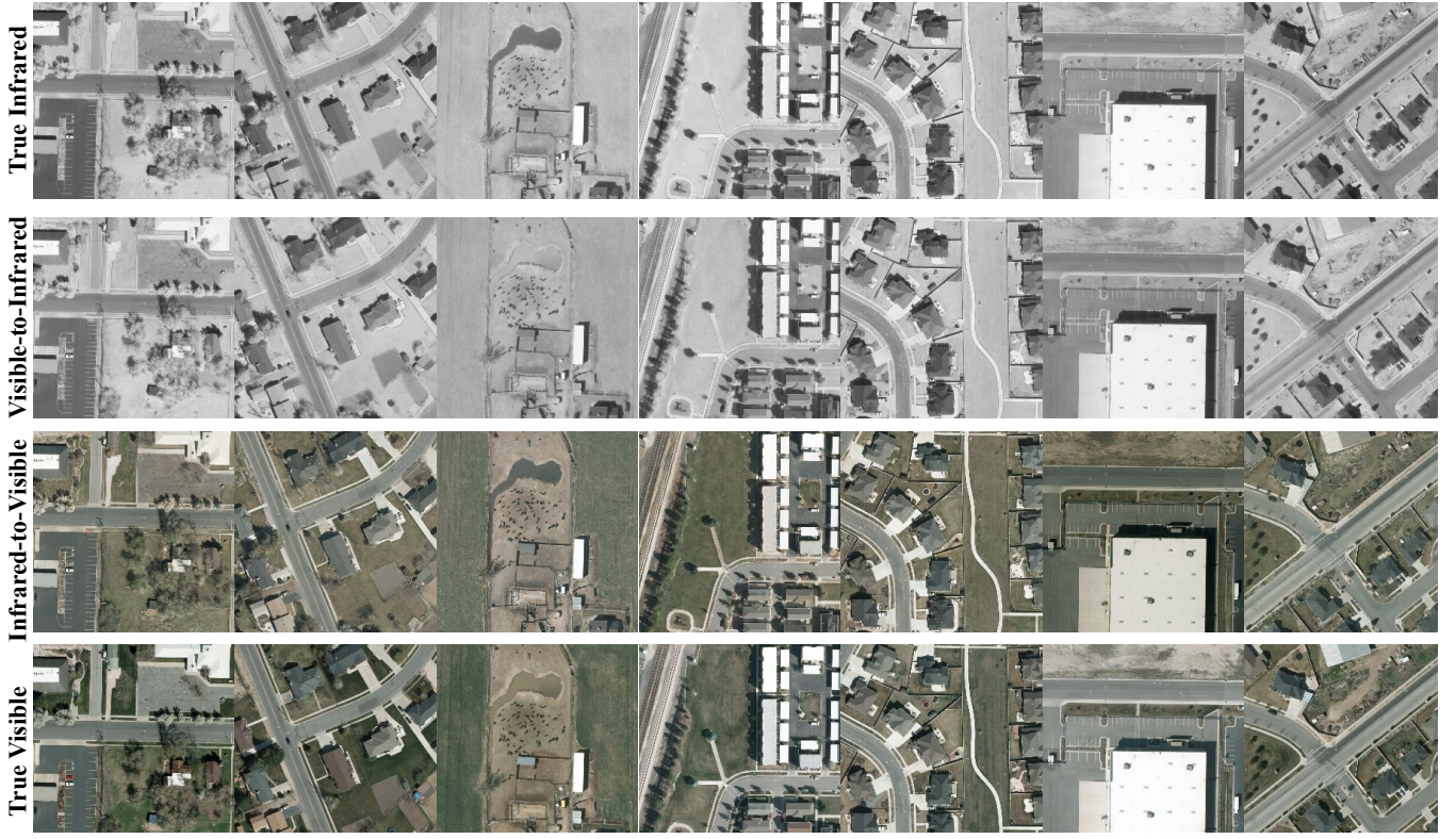
Figure 10: Modality translation results on the VEDAI dataset. The first row represents real infrared images, the second and third rows show generated infrared and visible images, respectively, and the fourth row represents real visible images.
