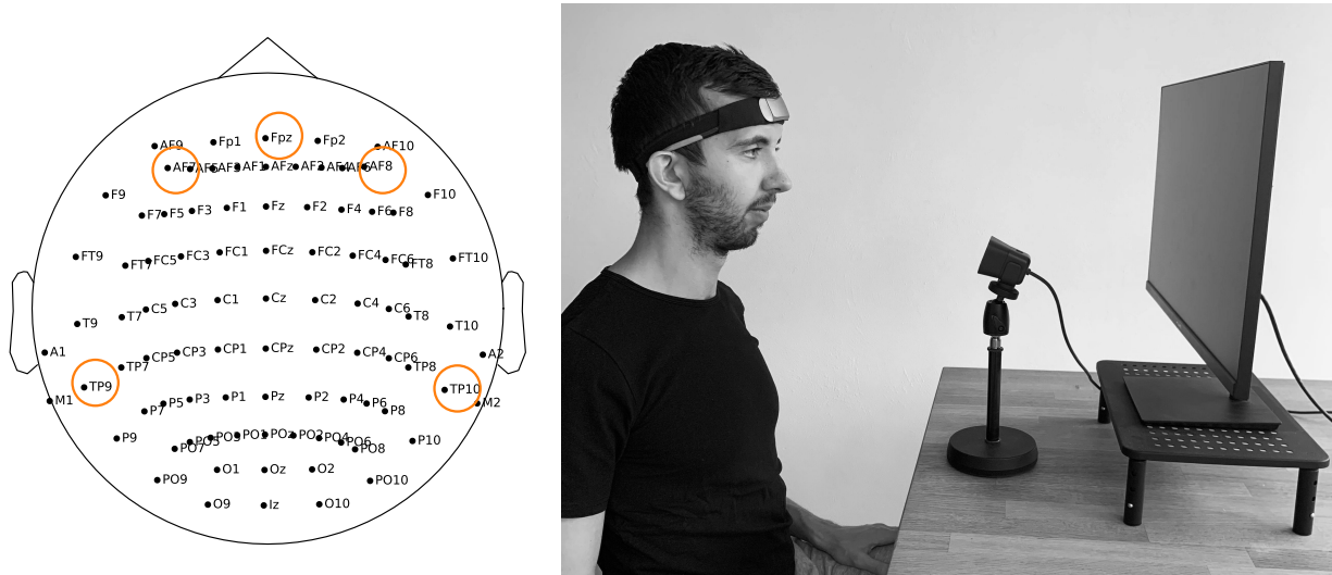
Figure 5: Left: Positions of electrodes of the Muse S 2 Headband in the 10-20 system. Right: Recording setup of the experiments. Consent was obtained for publication of the individual’s facial image.
