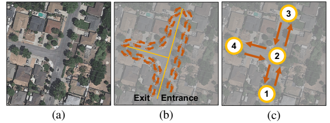
Figure 3: Maze wall follower approach to road polygon generation: (a) aerial view of a T-junction, (b) wall follower sequence, (c) resulting "empty" polygon (1→2→3→2→4→2→1).
