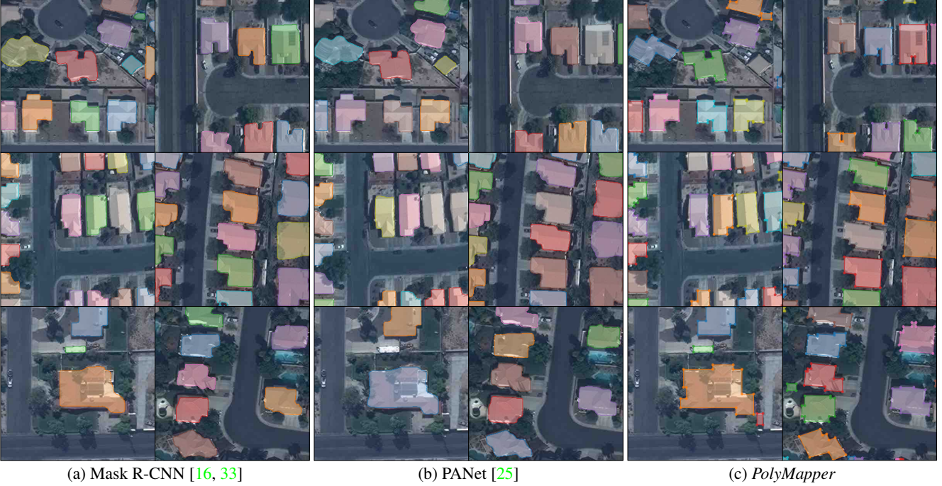
Figure 7: Building footprint extraction results on 4 example patches of the crowdAI dataset [33] achieved with (a) Mask R-CNN [16, 33], (b) PANet [25], and (c) PolyMapper . Note that results in (a) and (b) are images labeled per pixel whereas PolyMapper shows polygons, as well as vertices connected with line segments.
