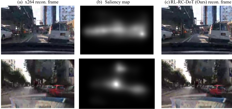
Figure 6. Saliency weighted PSNR results. (a) x264 reconstructed frame, (b) Saliency map of raw frame, extracted with [20] (c) RL-RC-DoT reconstructed frame. Notice that both RL-RC-DoT and x264 used the same target bit-rate
