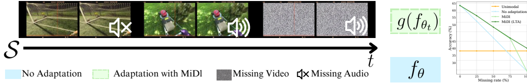
Figure 1: Test-Time Adaptation for missing modalities. The concept of test-time adaptation in the presence of missing data modalities focuses on a system where a stream of multimodal data is input, potentially lacking one or more modalities. Without adaptation, the pretrained model f_{\theta_0} may predict inaccurate labels due to incomplete data. With test-time adaptation, the model is dynamically adjusted using the adaptation method g , resulting in an adapted model f_{\theta_t} , designed to handle the missing modalities and improve over time. The graph on the right illustrates the performance of the non-adapted baseline (blue) vs. the model adapted with our proposed adaptation method MiDI (green) on Epic-Kitchens dataset. It shows the adaptation efficacy in maintaining higher performance levels despite the variability in modal-completeness, surpassing the unimodal performance (orange) for all missing rates.
