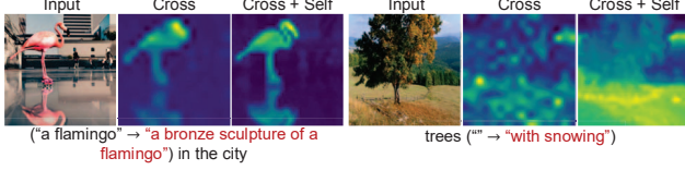
Figure 5. Refining cross-attention using self-attention [31] produces editing masks with higher contrast and sharper boundaries.
