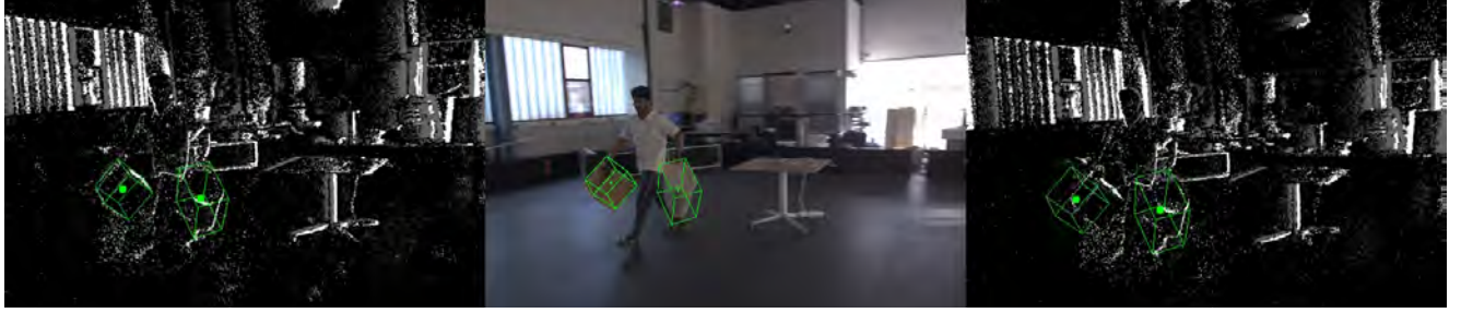
Figure 5. The figure displays the 6D pose annotations for two objects from our dataset of 16. Event images are generated by accumulating events over a 10 ms period.
