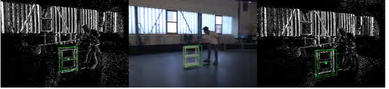
Figure 7. The figure shows 3D bounding box annotations that appear inaccurate in the RGB image due to jerky motion or sudden camera movements. We provide RGB images with improved annotations using a 100 FPS RGB camera. Event images are generated by accumulating events over a 10 ms period.
