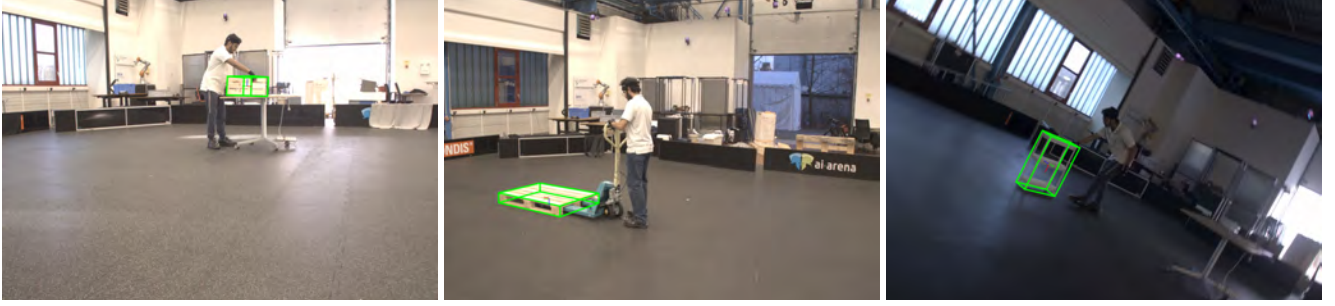
Figure 10. The figure demonstrates strong evaluation results with FoundationPose. It also highlights the diverse degrees of freedom present in the dataset. For example, the dataset includes variations in camera system height and angle, changing lighting conditions, and different human subjects. Additionally, glare from an open door adds another layer of complexity to the scene.
