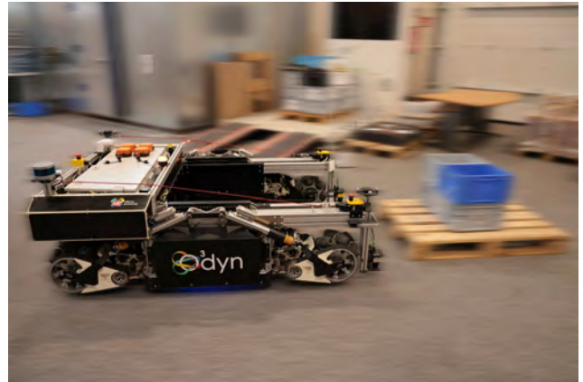
Figure 1. Mobile robot navigation speeds are continuously increasing. This figure shows O 3 dyn [27], an open-source outdoor robot platform capable of reaching speeds of up to 10 m/s. While the locomotion hardware supports these speeds, high-speed perception remains a bottleneck. Event cameras enable such robots to detect moving objects while navigating at high speeds. Additionally, 6D pose estimation with event cameras allows robots to execute grasps more quickly, improving overall efficiency in dynamic environments.
