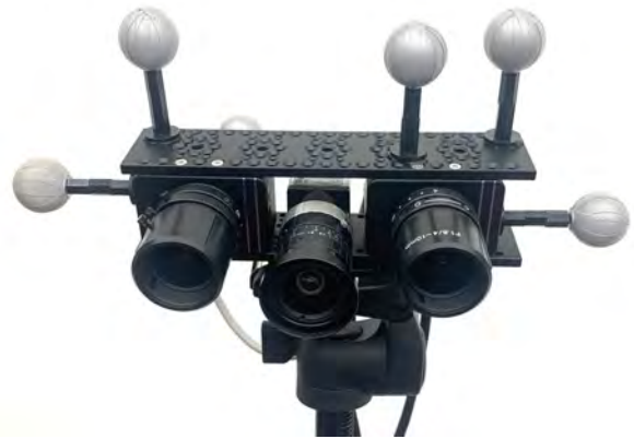
Figure 2. The camera system used for dataset recording, with the RGB camera at the center and the two event cameras positioned on either side. Six retroreflective markers are attached for precise motion capture.
