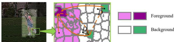
Fig. 3 Spatial cue illustration. White foreground and black background based on superpixel level. The dark purple superpixel accumulates sufficient differences from other ones, which is demonstrated by the orange solid lines. The green superpixels have a small scope of surrounding background. Orange dotted lines denote differences from other superpixels cannot contribute to the certain superpixel.
