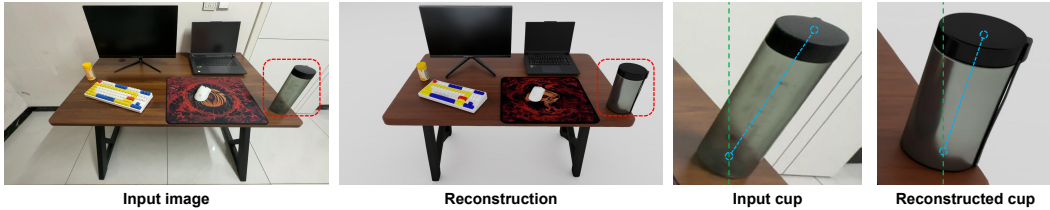
Figure 7: Residual projection misalignment. Despite the overall scene alignment, the reconstructed cup exhibits less projected tilt than the input cup. Red boxes identify the cups; cyan dashed lines indicate their projected axes, and green dashed lines indicate the image vertical.
