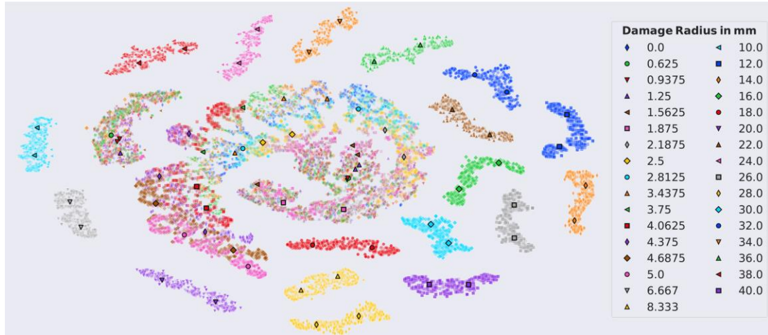
Fig. 2. 2D t-SNE embedding of synthetic data with two samples per debonding size selected by the CCU algorithm (marked by black border).
