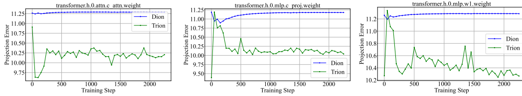
Figure 2: Projection errors for Dion and Trion for a few layers from the first transformer block on Llama-30M ( d = 640, r = 128 ).
