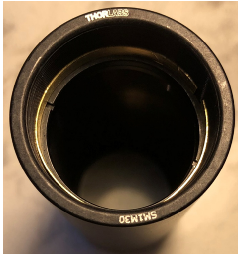
Fig. 6 A strip of brass is inserted first and rests on a retaining ring that serves as a lens spacer and seat.
