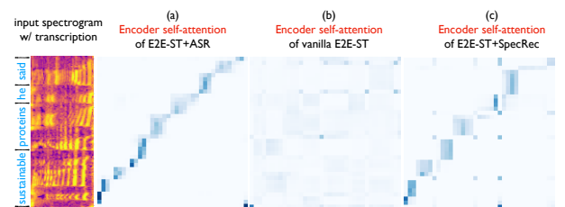
Figure 3: One head of the last layer self-attention comparison between different models. ASR MTL and SpecRec help the encoder learns similar self-attentions. See discussion in 4.1.
