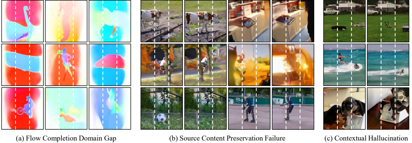
Figure 3. Key limitations of existing video outpainting approaches. (a) Flow completion domain gap : Flow completion networks trained for video inpainting struggle to generalize to video outpainting due to the substantially larger missing regions involved. Consequently, the predicted flow often suffers from bleeding around dynamic objects and fails to provide reliable motion estimates for regions far from the original content. (b) Source content preservation failure : Generation-based approaches often fail to preserve the original source content across frames when spatially extending video frames. As a result, visual content may disappear or fail to appear consistently in the generated regions, leading to temporal inconsistency throughout the video sequence. (c) Contextual hallucination : Due to the limited contextual cues available for video outpainting, generation-based methods may hallucinate semantically irrelevant or unrealistic content in the outpainting regions. Such hallucinations introduce visual artifacts and intra-frame inconsistency.
