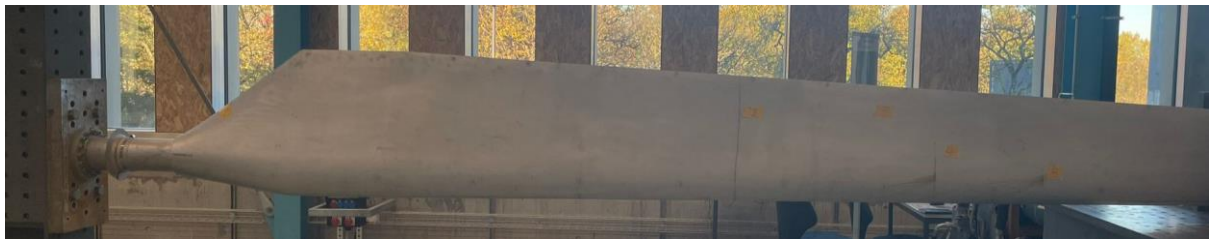
Figure 1. The blade from the Aventa AV-7 "Light Wind Turbine", that was sold and copyrighted under the Leichtwindanlagen© name, mounted on a sturdy wall in Bauhalle, ETH Zurich. Low pressure (LP) side.
