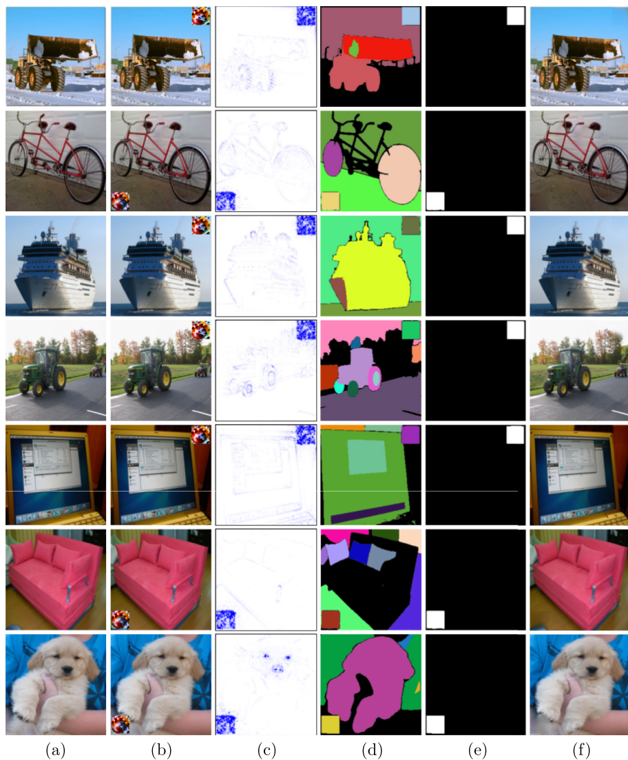
Fig. 16 The full process of defending against a Generative Dynamic Patch Attack. (a) A benign image has a patch applied to it to become an (b) attacked image. PATCHOUT defends the image by using (c) attribution analysis and (d) image segmentation to find the (e) patch location. Finally, the patch location is inpainted, resulting in the (f) restored image
