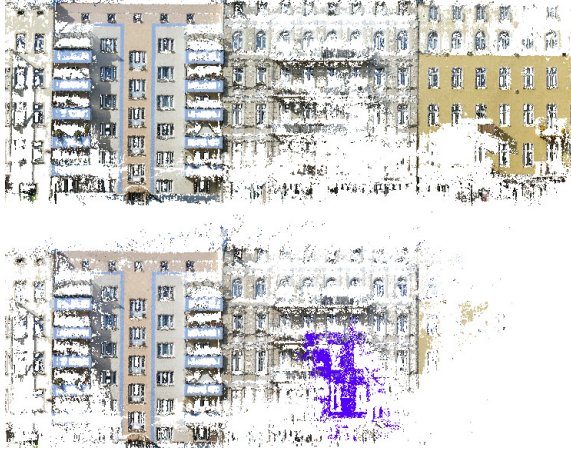
Figure 5. Dense point clouds after applying Proposed-Filter (top) and Filter-by [16] (bottom) methods. The purple points indicate wrongly reconstructed points.
