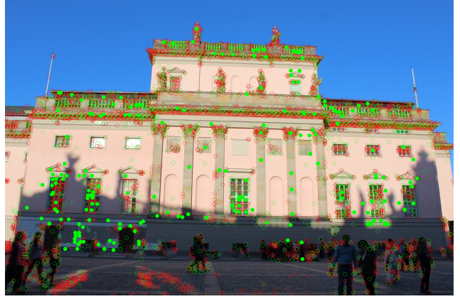
Figure 3. Image containing repetitive patterns, homogeneous areas and pedestrians. Initially detected keypoints are depicted in red, predicted as matchable in green, and the finally matched as filled circles.
