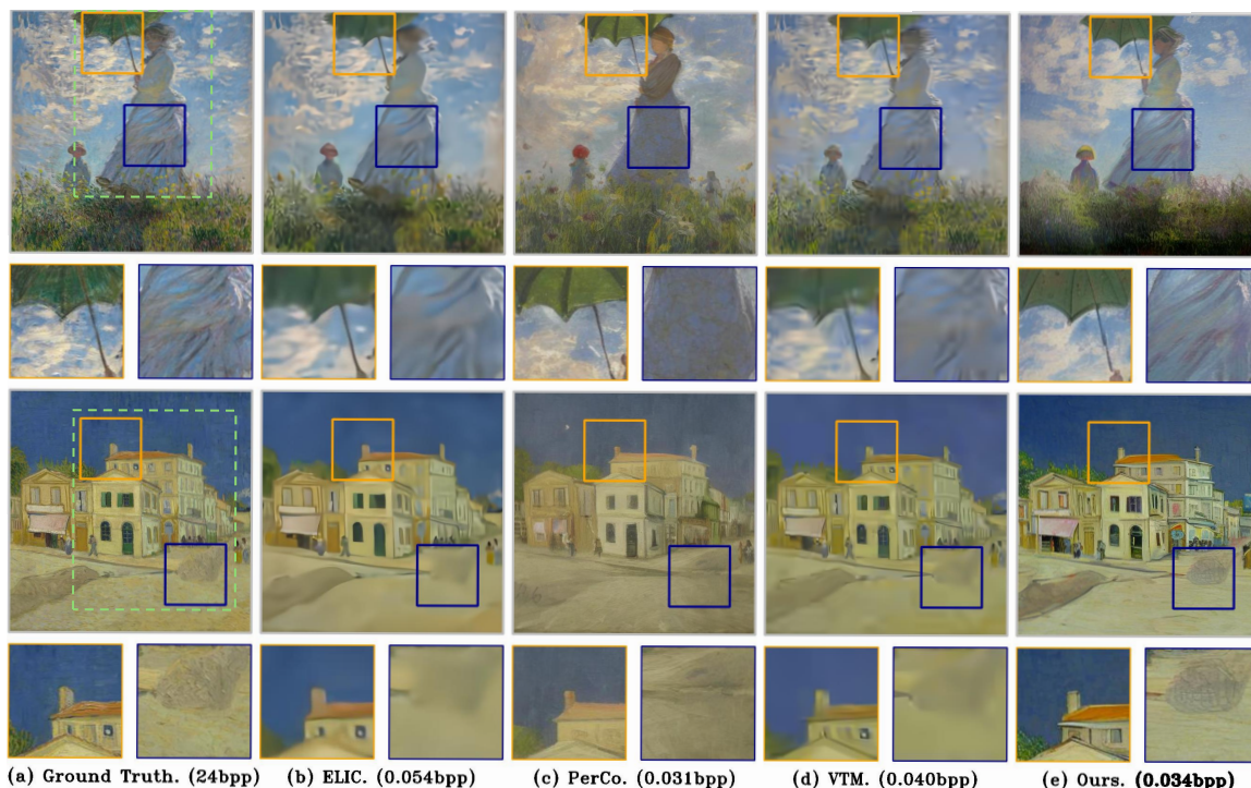
Figure 1. Visual comparison of decoded images. (a) Original images with the user-specified RoI area highlighted by a green dashed box. (b) VAE compression method cannot achieve extreme-low bitrate considering distortion optimization. (c) PerCo sacrifices the consistency of key areas to obtain realism at extreme-low bitrate. (d) Traditional encoders have severe blocking effects at extreme-low bitrate. (e) The proposed method maintains the overall advanced perceptual quality and maintains the consistency of key areas.
