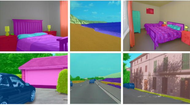
Figure 7. Segmentation results of COSNet on ADE20K validation set. We notice that our framework can effectively segment the objects by using boundary information.
