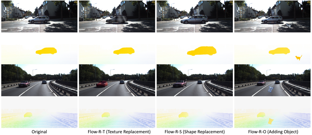
Figure 1. Samples of Flow-R. Original and modified images (Row 1 and 3), ground truth optical flows (Row 2 and 4) are shown. The first column displays the original data from the KITTI dataset. The second column shows the data with the texture of the main object of car replaced. The third column shows the data with the shape of the main object rescaled. The fourth row presents the data with an unseen object added.
