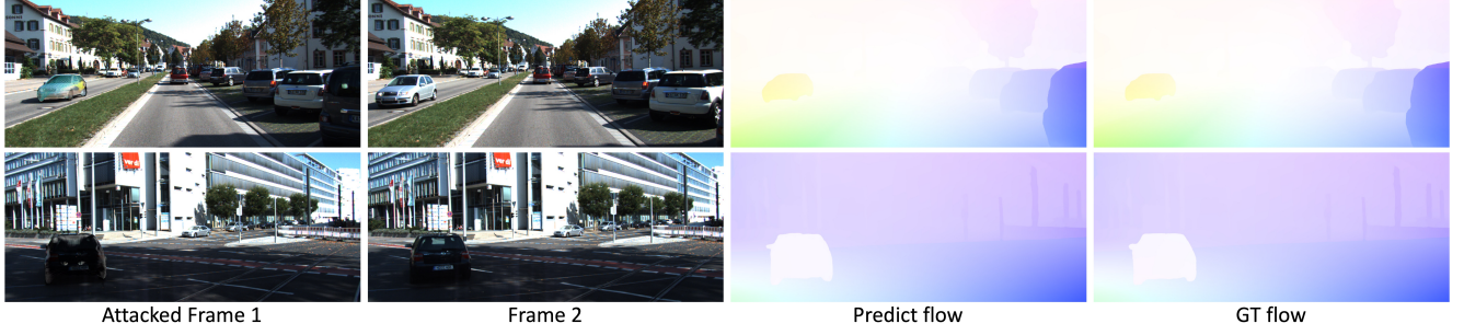
Figure 3. Texture Attack. The texture of the main object (car) in the first frame is replaced, while the second frame remains unchanged. The resulting optical flow is similar to that derived from the original images.
