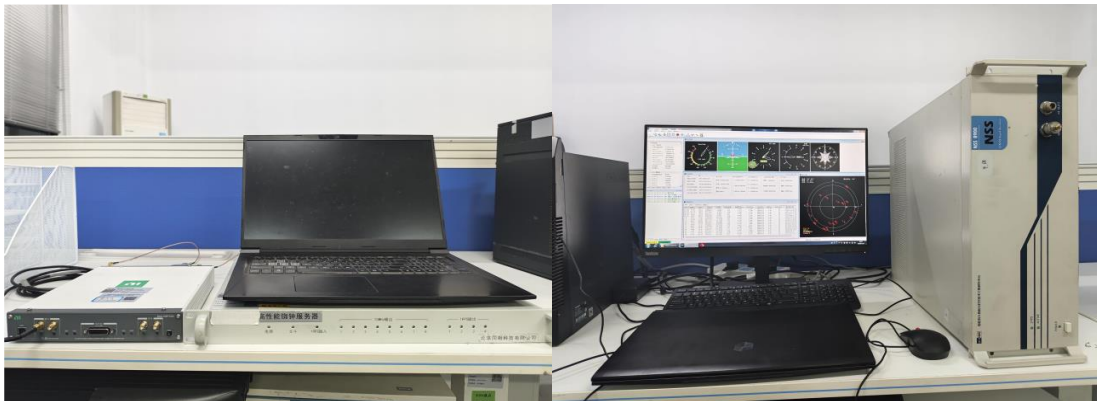
Fig. 18 Equipment Configuration for the Test. The left panel includes the receiving equipment-comprising the receiving device, receiving computer, software radio, and rubidium atomic clock-while the right panel shows the transmitting equipment, which consists of the transmitting computer and NSS8900.
