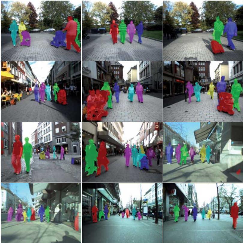
Figure 5.6.: Exemplary segmentation results, showing that the proposed approach is able to correctly segment the blobs of objects into individuals.
