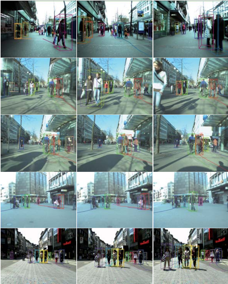
Figure 3.11.: Results from our tracking framework on the BAHNHOF, SUNNY DAY, JELMOLI and SHOPPING sequences.
