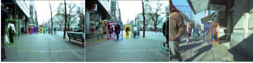
Figure 4.9.: Examples demonstrating our approach’s capability to continue tracking persons close to the camera and/or the image borders, where object detection is no longer applicable.
