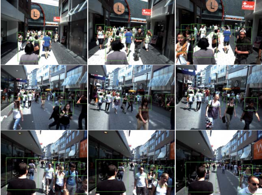
Figure 6.5.: Detection results, showing that our detector detects most of the present pedestrians close to the camera. The maximum range for this test was set to seven meters.
