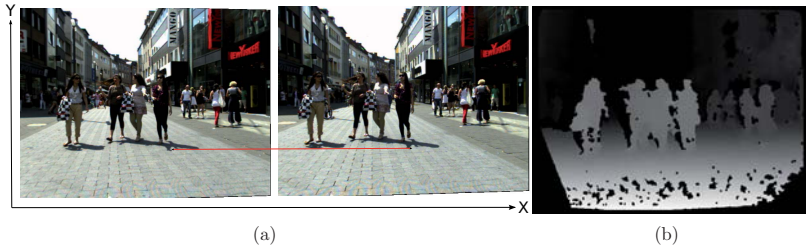
Figure 3.5.: (a) A rectified stereo pair, where the red line shows that the corresponding points have the same y-coordinate. (b) Corresponding disparity image obtained with the approach from (Geiger et al. , 2010).
