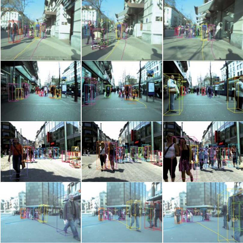
Figure 9.9.: Result images showing pure tracking-before-detection results. (First row) SUNNY DAY sequence. (Second row) BAHNHOF sequence. (Third row) SHOPPING sequence. (Fourth row) JELMOLI sequence. Note that no pedestrian classifier was applied here. The results further corroborate that the point cloud classifier presented in Chapter 5 classifies the points from elevated structures correctly as no tracks are extracted on the buildings.
