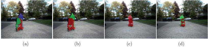
Figure 5.5.: Failure cases in segmentation using the classical ROI extraction approach. (a) Exemplary result of segmentation using the classical ROI generation approach, clearly showing over-segmentation. (b) the same as (a), but using the proposed accumulated ROI extraction process. (c) Classical ROI extraction approach, clearly showing under-segmentation. (d) the same as (c), but with accumulated ROI extraction, showing the correct segmentation of pedestrian and object.
