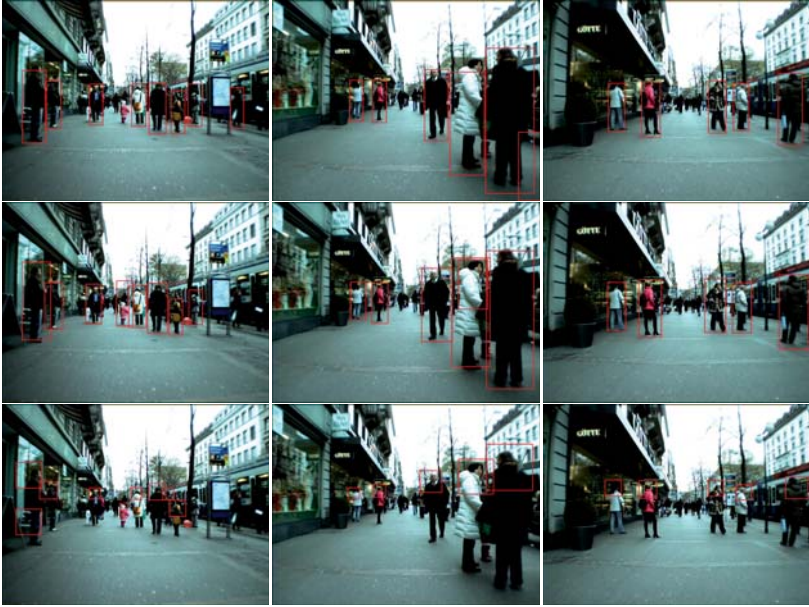
Figure 3.1.: Example results of the pedestrian detectors on the BAHNHOF sequence. First row corresponds to the output of the detector proposed by (Felzenszwalb et al. , 2010b). Second row (Sudowe and Leibe, 2011) and the last row shows the output from our upper body detector presented in Chapter 6.
