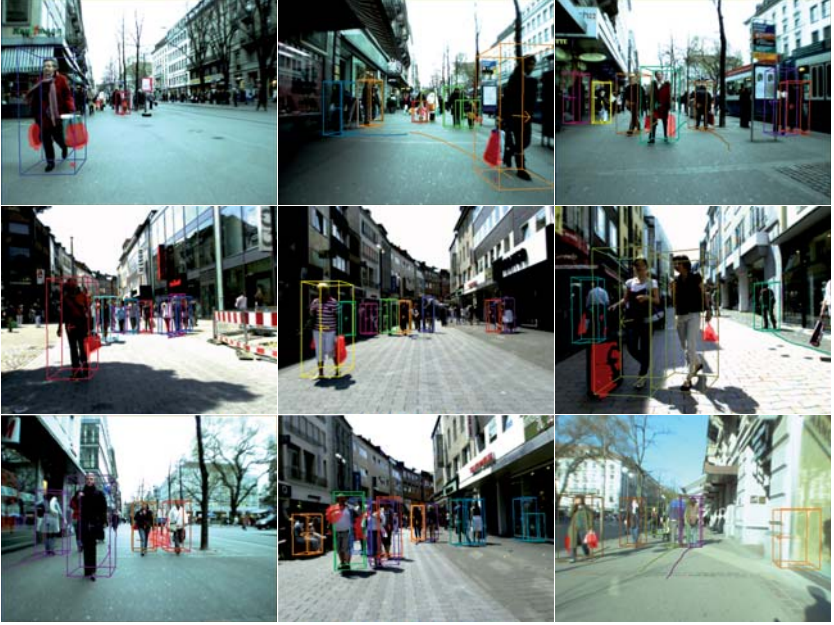
Figure 8.6.: Carried item detection results (in red). The bottom row shows some failure cases which are caused by depth smoothing, excessive body proportions, and unusually wide clothing.
