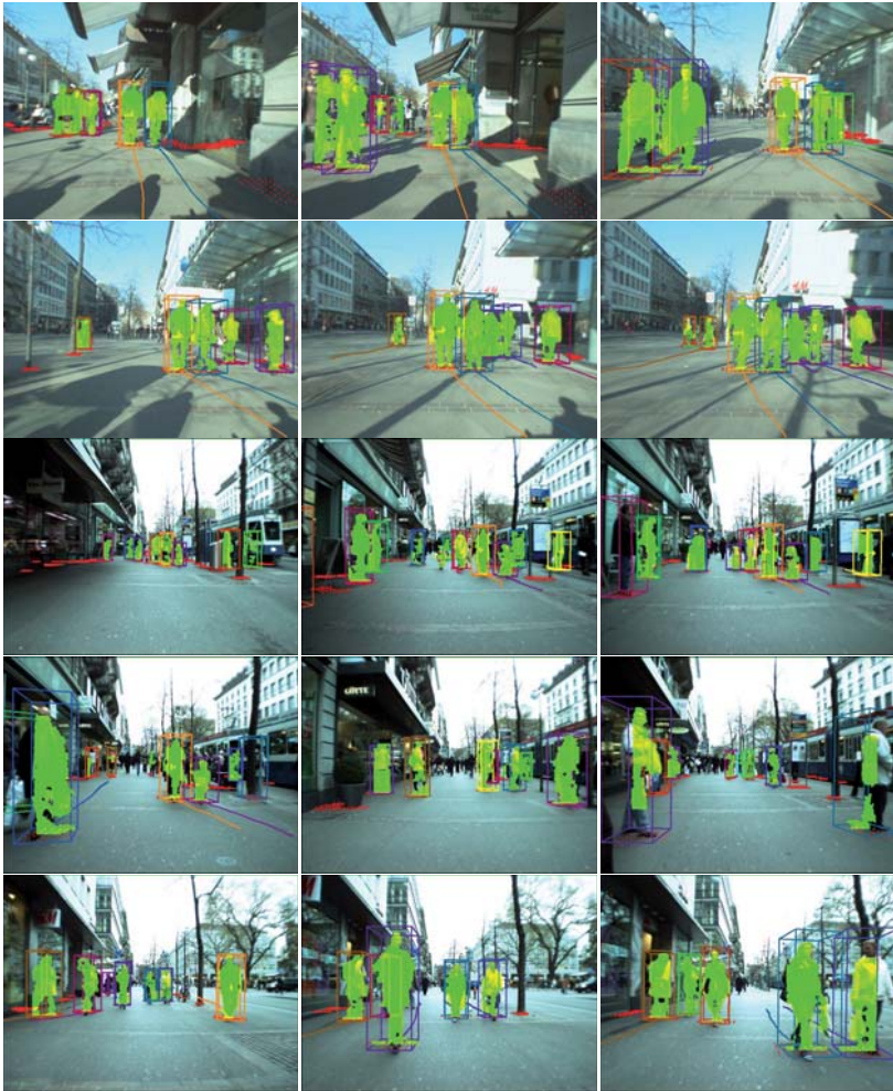
Figure 4.19.: Example results on the test sequences SUNNY DAY and BAHNHOF. The green overlay inside the box corresponds to the depth information used for computing the ROIs. Red points on the ground plane represent the ROI foot points.
