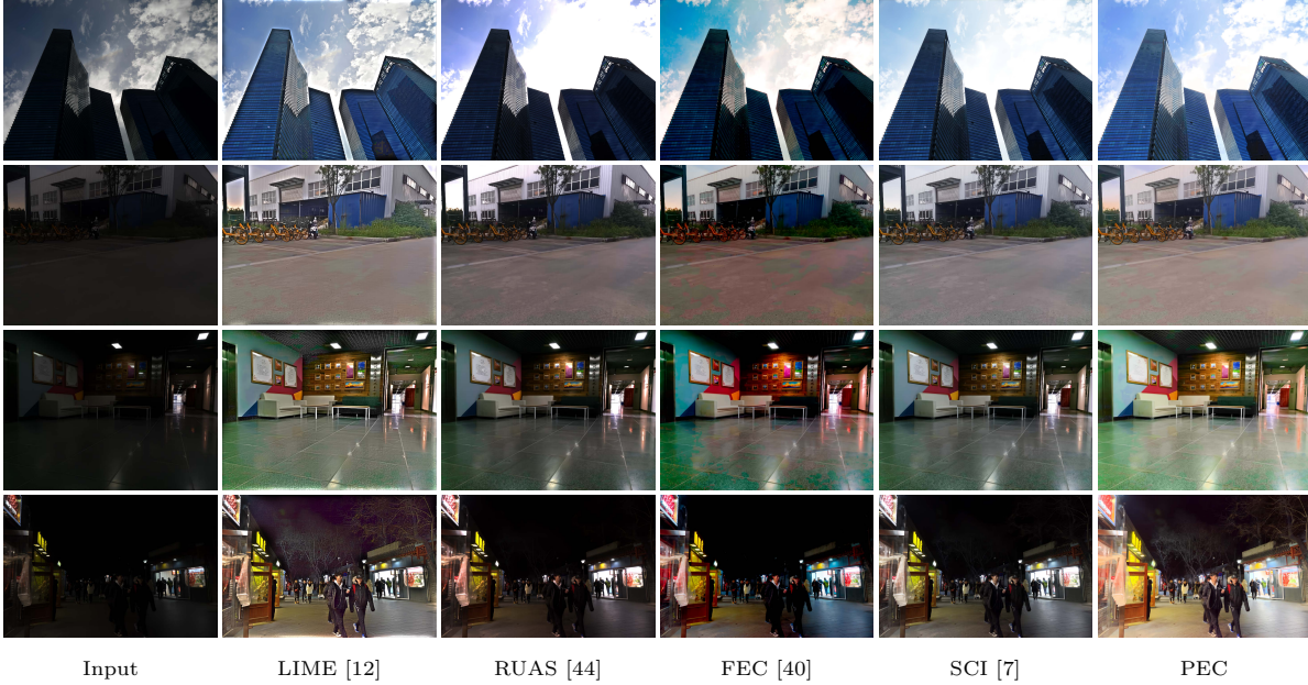
Figure 8 Visual comparison of under-exposure scenarios with noise. Except for the input, all correction results were processed by denoising (SCUNet) for better visualization.
