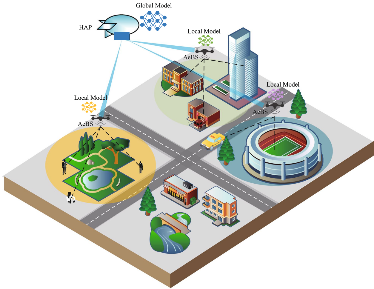
Fig. 1 HAP-assisted multi-AeBS deployment architecture
