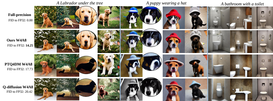
Fig. 7: Comparison between the quantized models and the full-precision model. Use Stable diffusion 512 x 512. Relaxation proportion \tau = 0.20 .
