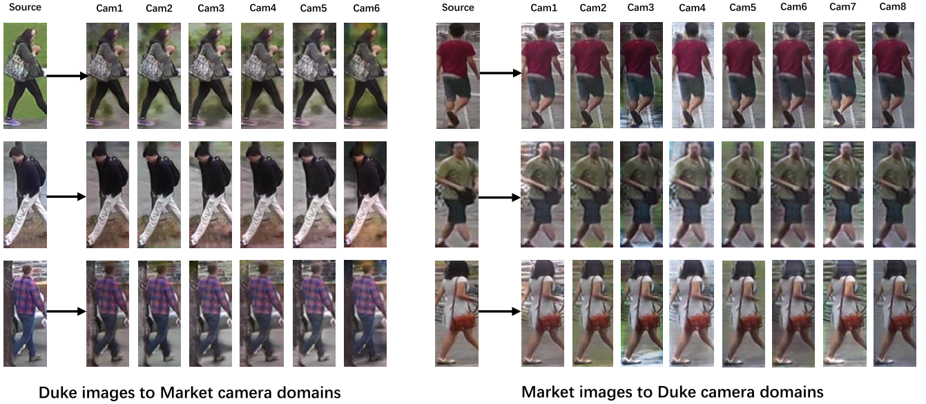
FIGURE 4. Visual examples of images from source domain to target camera domains translation. The left seven columns map DukeMTMC-reID to Market-1501 six camera domain styles. The right nine columns map Market-1501 to DukeMTMC-reID eight camera domain styles.
