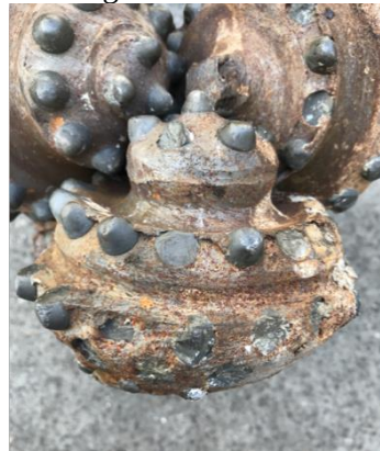
Fig.9 Photos of a broken tooth in actual working condition
