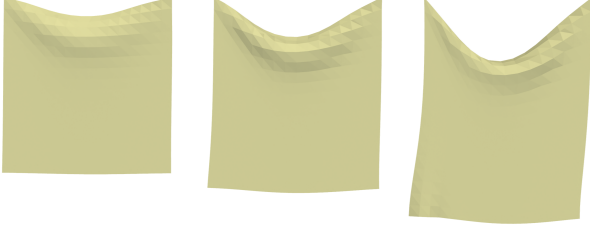
Figure 13. We drape three pieces of cloth with different extensible limit. From left to right, we use (\bar{l} - l)/l = 0.1, 0.2, 0.4 .
