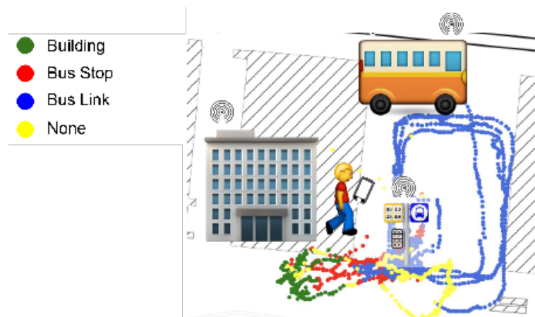
Figure 2 - BLE network - BLE beacons installed on bus, bus stop and building. The figure shows an example of GPS trajectory automatically labeled with BLE proximity.
