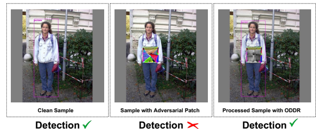
Figure 1. Demonstration of Adversarial Defense with ODDR [Task: Person Detection (Object Detection sub-task), Model: YOLOv4 [2], Patch: AdvYOLO [38], Dataset: INRIA [12]].
