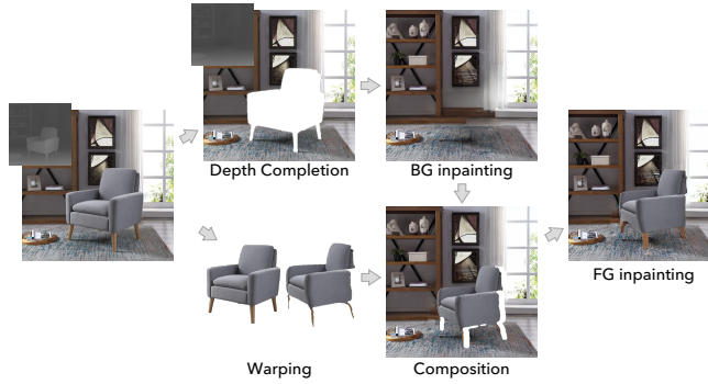
Fig. 3: Illustration of our view synthesis stage with a layered, diffusion-based generative inpainting scheme.
