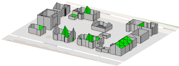
Figure 9: The calculated SharedWall featured for building in a closed construction
