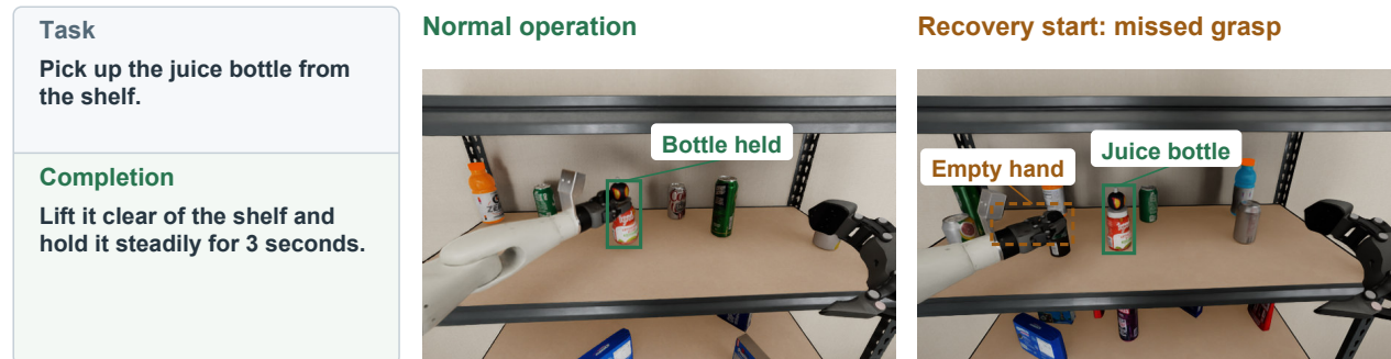
Figure 40. Failure Recovery: normal shelf pickup (left) and a missed-grasp state (right).
