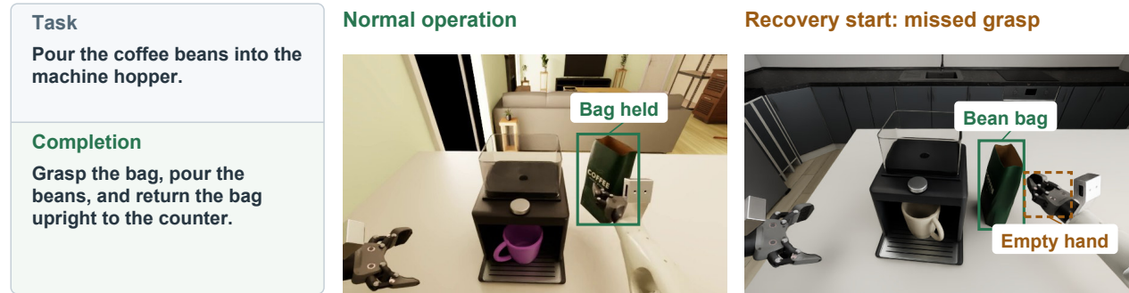
Figure 41. Failure Recovery: normal bean-bag pickup (left) and a missed-grasp state (right).
